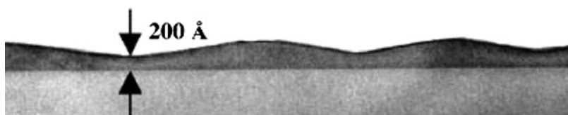
Figure 13.5. Cross-sectional TEM of a \text{Si}_{0.8}\text{Ge}_{0.2}/\text{Si} layer deposited at 630^\circ\text{C} . From Phys. Rev. B 59 , 1990(1999) with permission. © 1999 American Physical Society.
